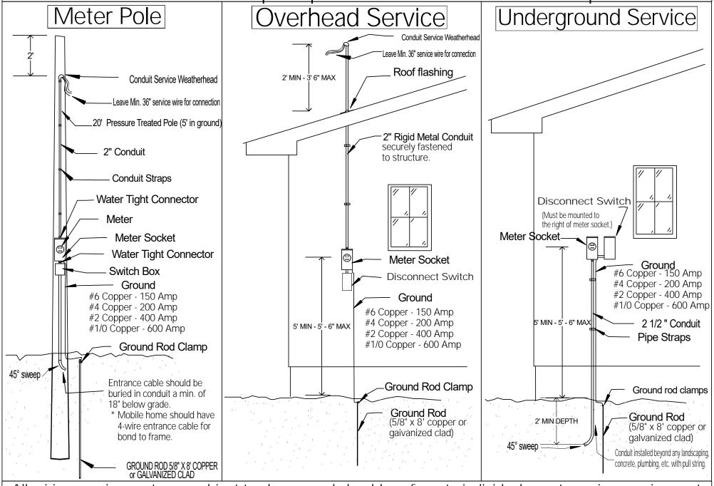
All wiring requirements are subject to change and should conform to individual county zoning requirements All items pictured are to be provided by the consumer except for the meter. Diagrams above meet minimum requirements of the 2011 National Electric Code.
